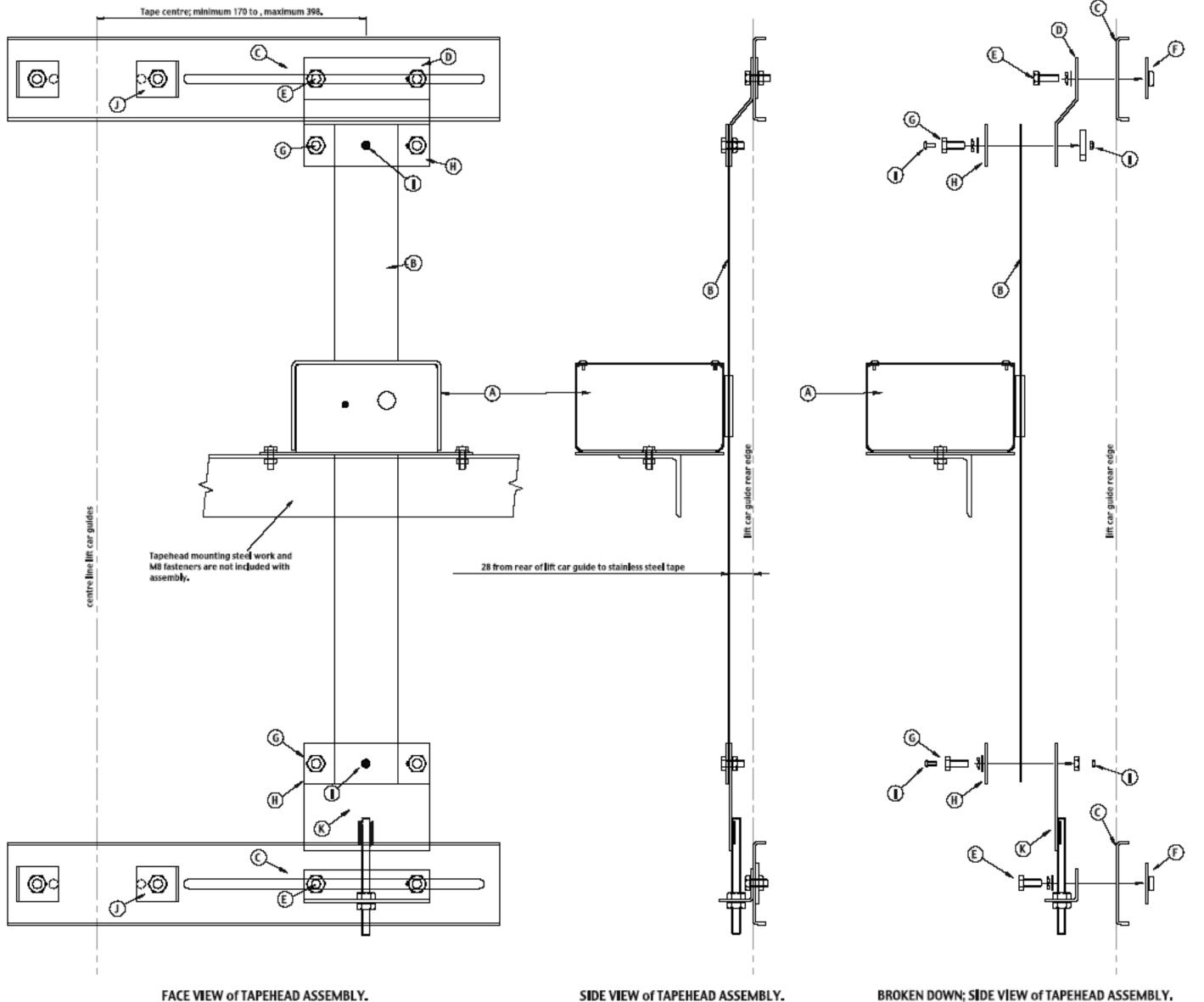
Lester Control System Ltd, 7 channel detector / tapehead unit, with floating head. O/A dimensions: 178W x 110H x 172L. Mounted on to a 3mm thick. Garvanised plate 254L. x 72W, with 2No 50 x 9 car mounting slots
