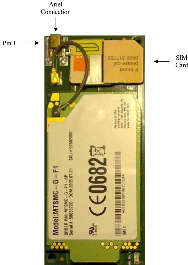
The GSM (Global System for Mobile Communications) modem option allows the lift to connect via a wire free connection, either using dialup internet, or a dialup 1-1 operation.
