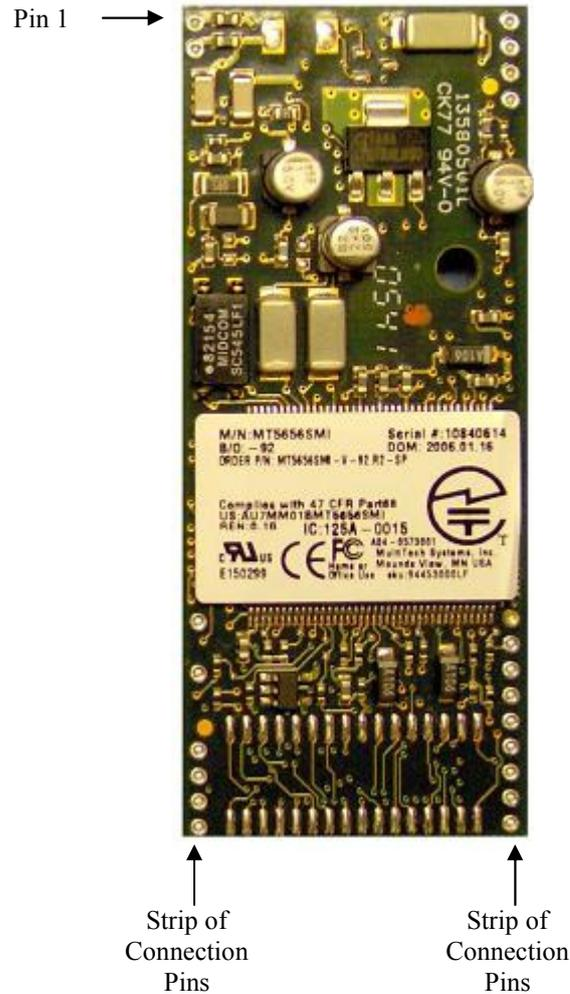
The PSTN (Public Switched Telephone Network) modem option allows the lift to connect via a standard telephone socket, either using dialup internet, or a dialup 1-1 operation.
