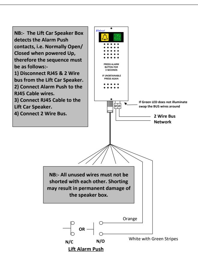
Note:- The RJ45 Cable is supplied with the unit. However, if any other RJ45 cable to be used for the unit, the plug must be made as per the above drawing. Incorrectly made plug will result in damaging of the unit and will violate warranty terms.
