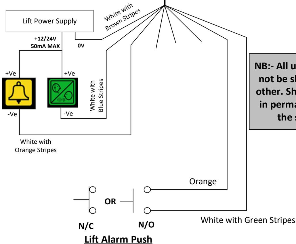
**NB:-** All unused wires must not be shorted with each other. Shorting may result in permanent damage of the speaker box.
