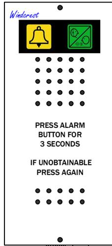
If Green LED does not illuminate swap the BUS wires around
