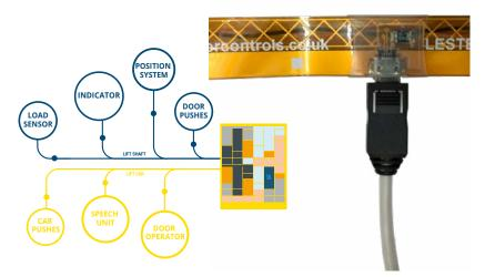
The Flexibus (Click & Connect) offers a variety of lift shaft features to allow quick set-up. The system features a revolutionary bus design which offers flexible power and data. Connections are made to low voltage shaft equipment, via low profile "locking" mini connectors. Fuse protection is provided per landing node whilst the fully screened data lines protect against outside interference.
