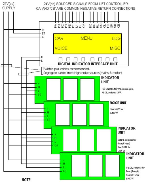
LINK 'A' is supplied connected on one pin only for all Indicator units. LINK 'A' must be fitted between both pins for last unit in communications run only (car & landing furthest from controller). Other units have LINK 'A' on one pin only.
